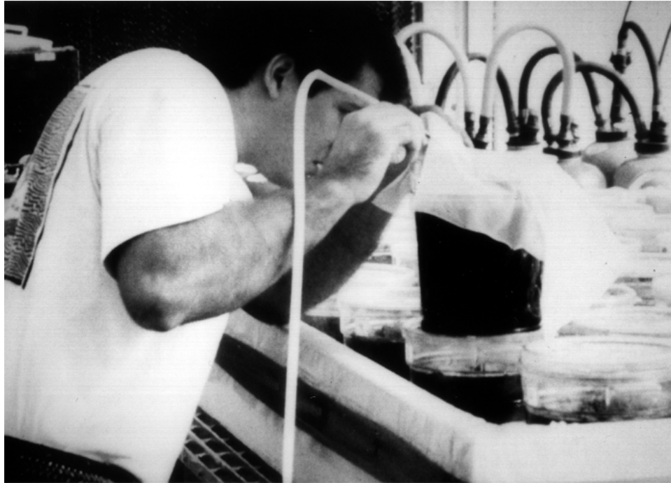
Figure 6. When adults emerge they are removed from the larval containers using an aspirator attached to a vacuum pump
