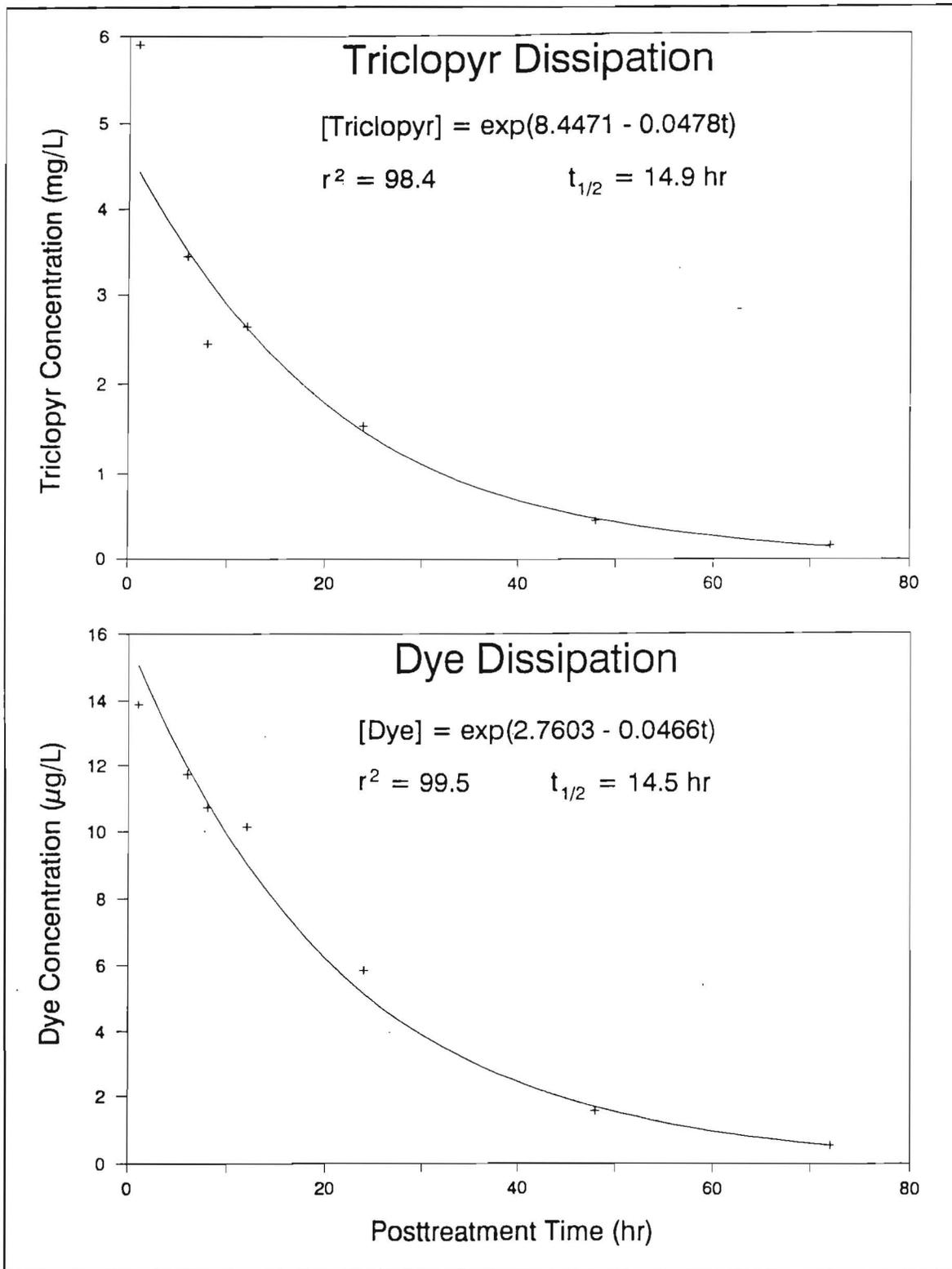
Figure 8. Dissipation of triclopyr and dye in upper portion of water column in river treatment (RT) plot following application of Garlon 3A and rhodamine WT, Pend Oreille River, Washington (Lines represent calculated dissipation curves using an exponential model, and symbols represent actual values)
