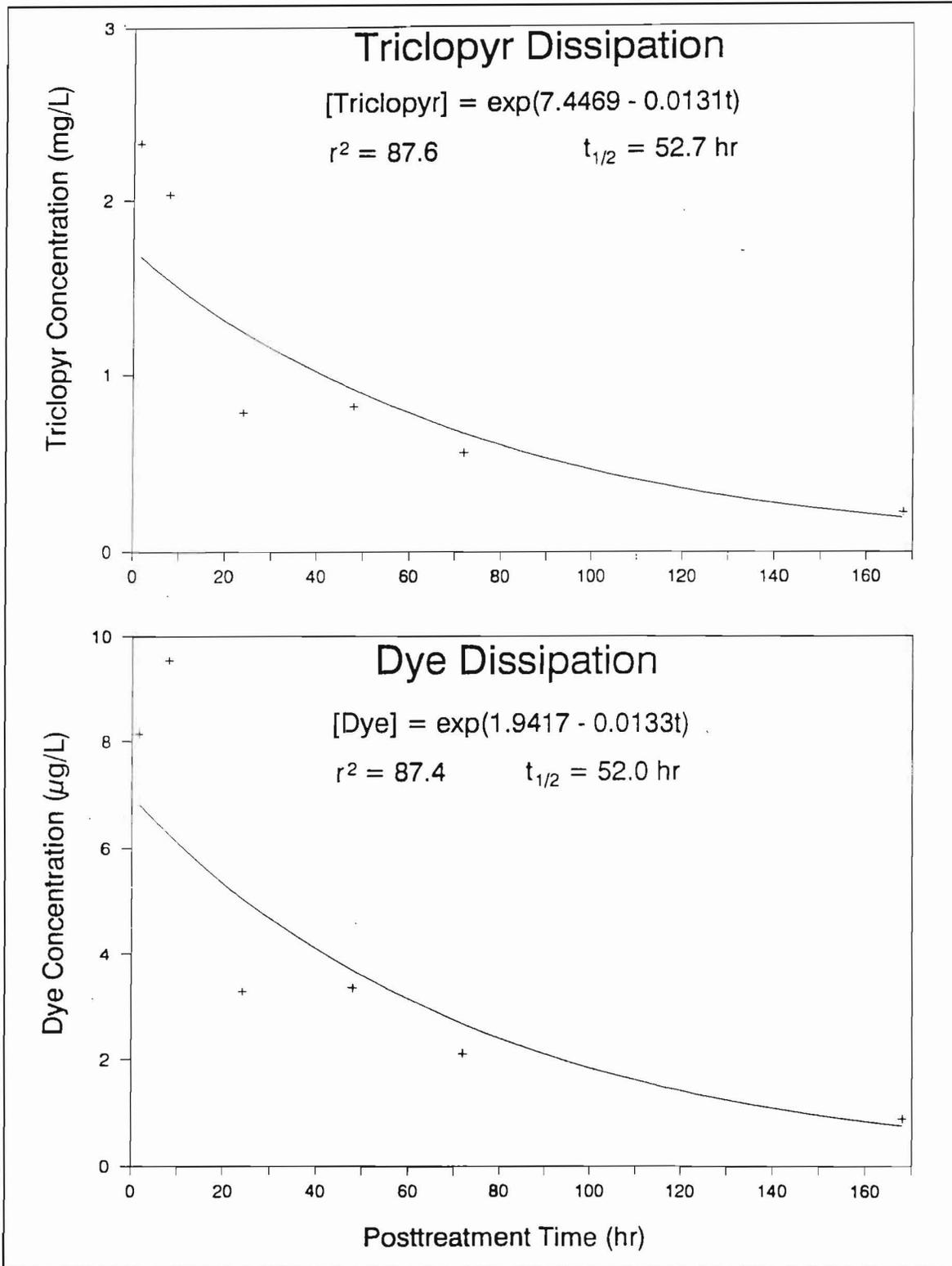
Figure 11. Dissipation of triclopyr and dye in cove treatment (CT) plot following application of Garlon 3A and rhodamine WT, Pend Oreille River, Washington (Lines represent calculated dissipation curves using an exponential model, and symbols represent actual values)
