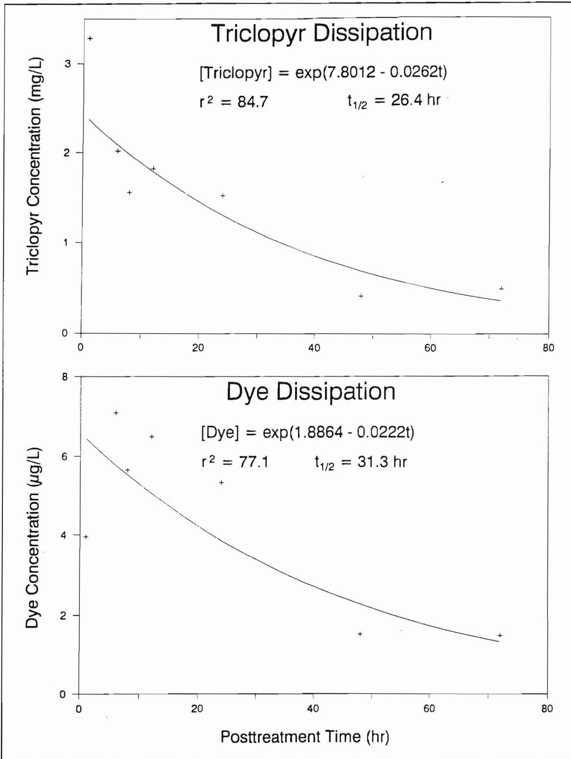
Figure 9. Dissipation of triclopyr and dye in lower portion of water column in river treatment (RT) plot following application of Garlon 3A and rhodamine WT, Pend Oreille River, Washington (Lines represent calculated dissipation curves using an exponential model, and symbols represent actual values)
