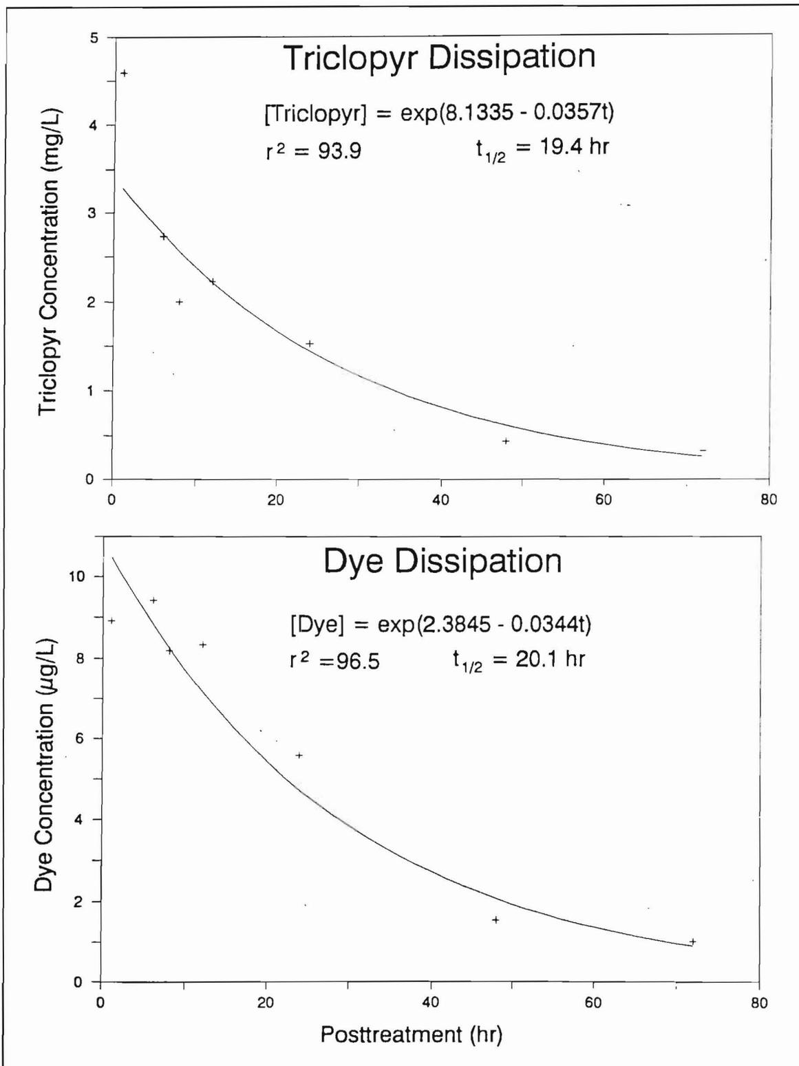
Figure 7. Dissipation of triclopyr and dye in river treatment (RT) plot following application of Garlon 3A and rhodamine WT, Pend Oreille River, Washington (Lines represent calculated dissipation curves using an exponential model, and symbols represent actual values)
