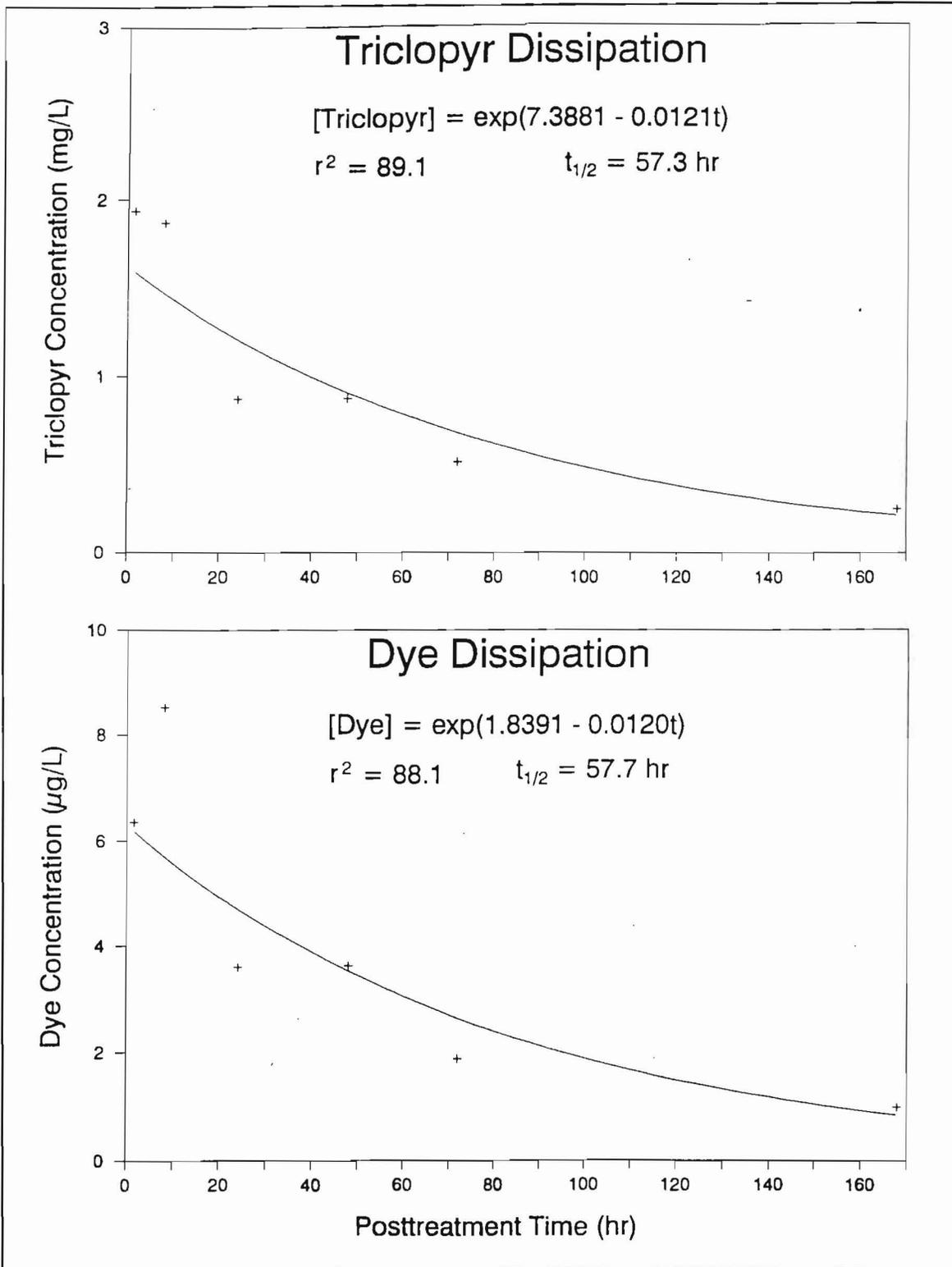
Figure 13. Dissipation of triclopyr and dye in lower portion of water column in cove treatment (CT) plot following application of Garlon 3A and rhodamine WT, Pend Oreille River, Washington (Lines represent calculated dissipation curves using an exponential model and symbols represent actual values)
