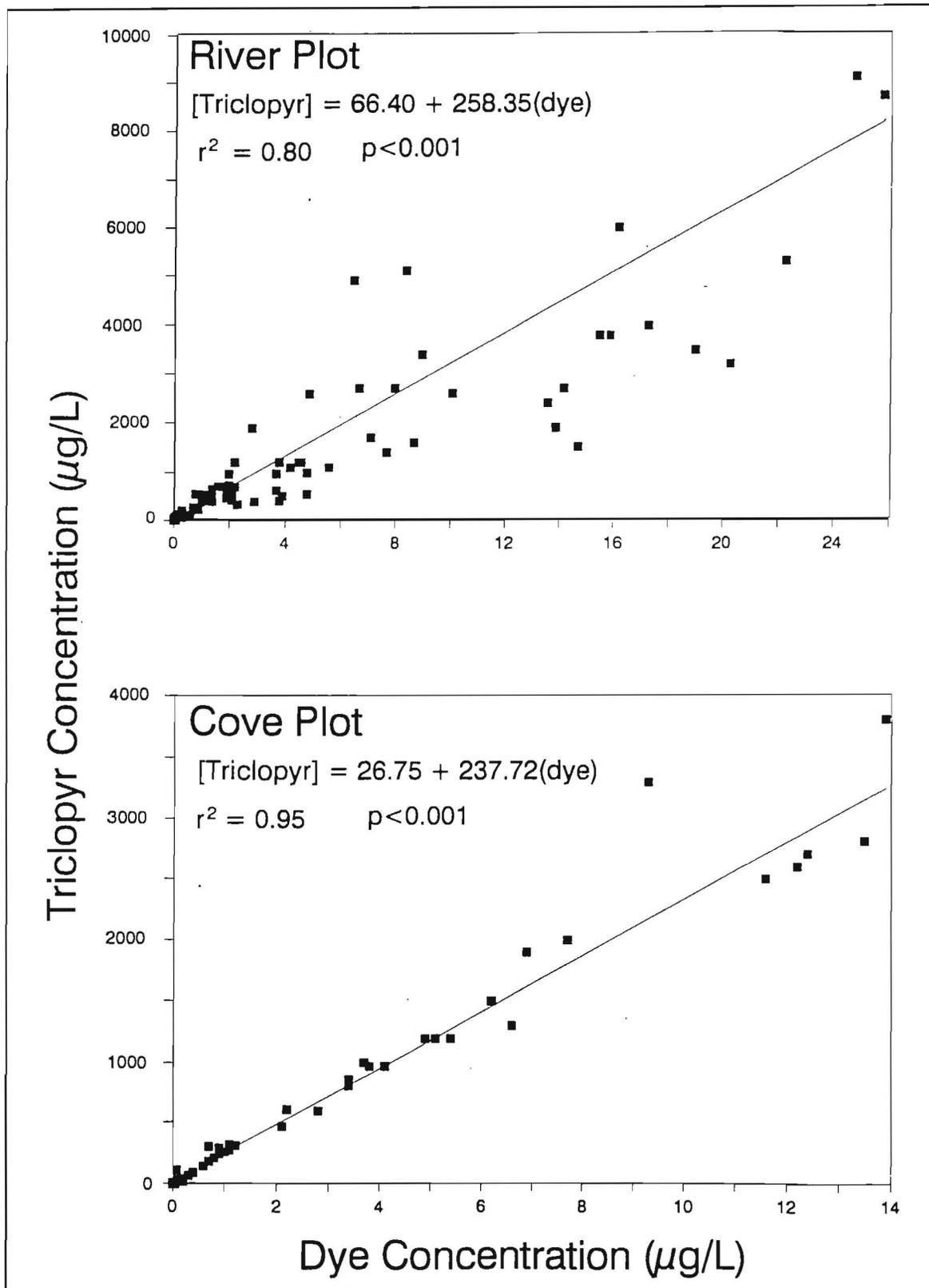
Figure 10. Correlations of dye and triclopyr following application of Garlon 3A and rhodamine WT to plots on Pend Oreille River, Washington
