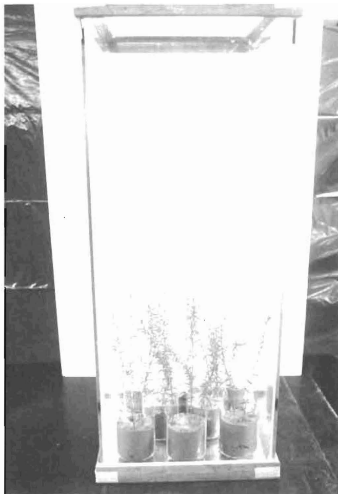
Figure 4. Hydrilla aquarium assay unit showing uninoculated hydrilla sprigs planted in beakers
