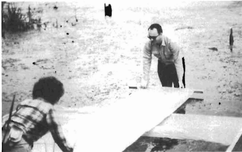
Figure 6. Field team placing reference markers to establish ground control on Lake Seminole
