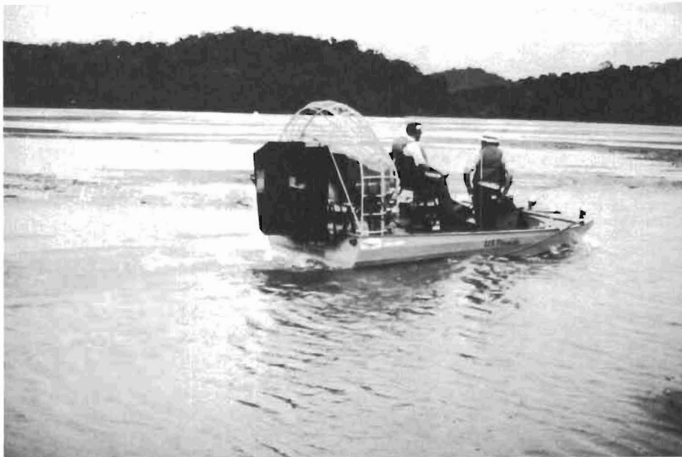
Figure 5. Application of fluridone 4AS formulation using spray pump and weighted trailing hoses
