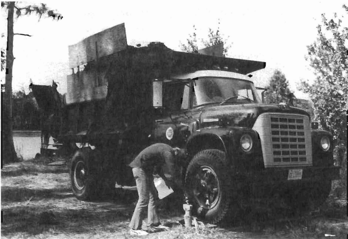
Figure 5. Weighing a loaded truck to determine weight of harvested plant material. The scale is the Hiway Load-o-Meter, Type A, load range 0 to 20,000 lb, manufactured by the Black and Decker Co.
