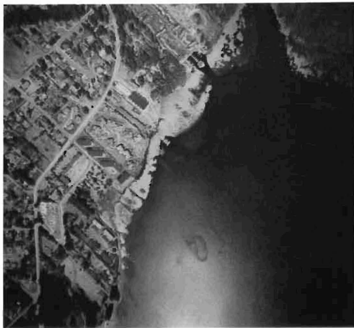
Figure 1. Example 1:5000-scale photograph of emergent plants using false color infrared film with filter
