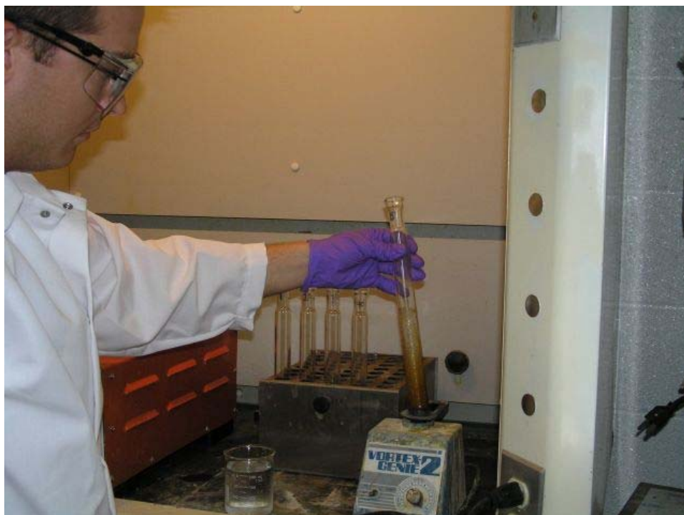
Figure 6. Setup for block digests of plant tissue for analysis for N, P, and K.
