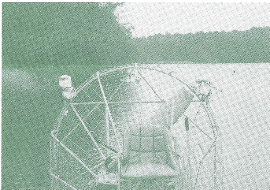
Figure 4. Two types of GPS antennas mounted on the cage of an airboat
