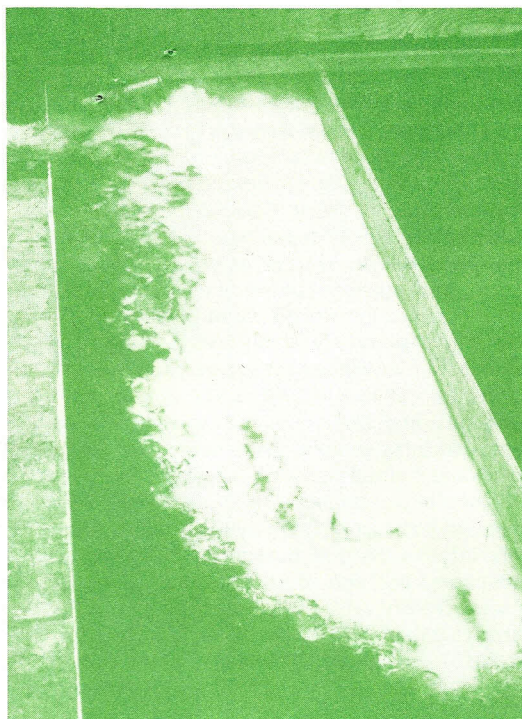
Figure 4. Milky consistency of a noninvert mixture
